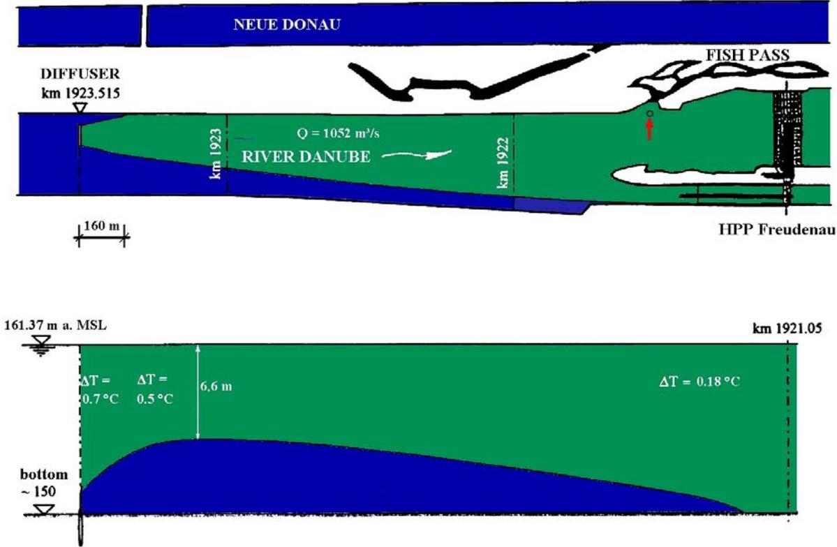
Fig.5: cooling water plume simulated by CORMIX for a discharge of 17.2 m<sup>3</sup>/s and a Danube flow rate of Q = 1052 m<sup>3</sup>/s
