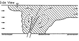
b) Surface Impingement with Buoyant Upstream Spreading d) Surface Impingement with Local Vertical Mixing, Buoyant Upstream Spreading and Restratification
